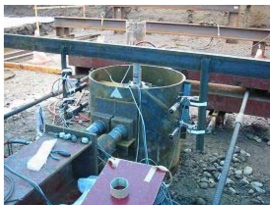
Figure 2 Horizontal load test set-up at Kiusu
