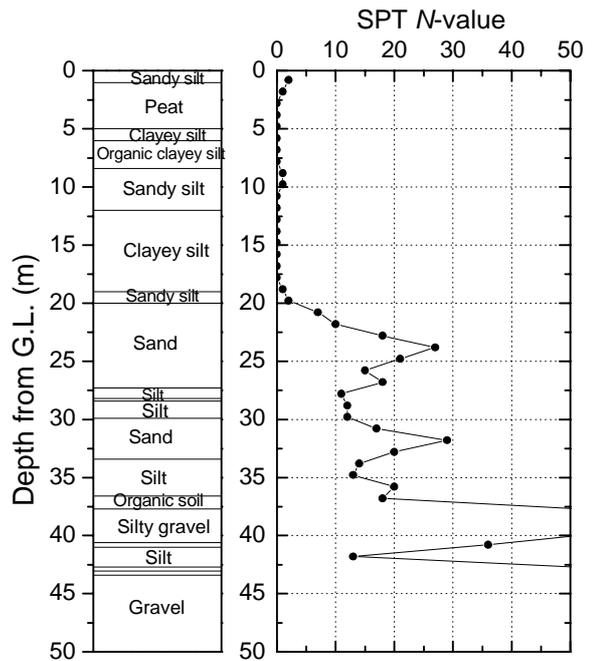
Figure 7 Profiles of soil layers and SPT  $N$ -values of the original ground at Shinotsu site
