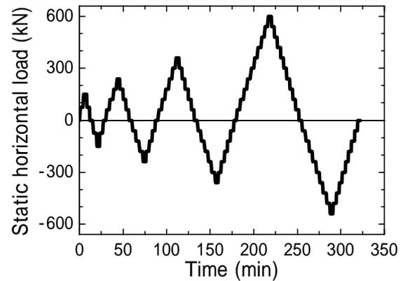
Figure 2 Loading procedure in horizontal load test
