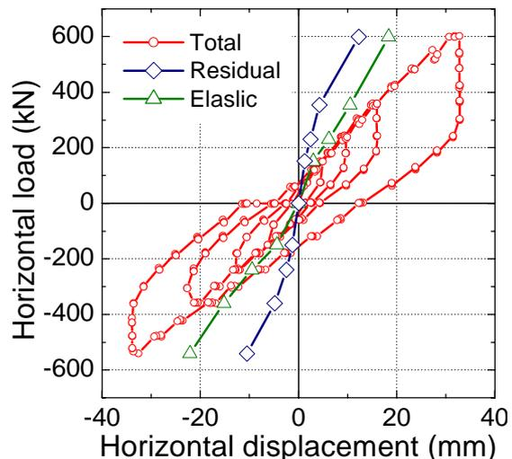
Figure 4 Horizontal load vs horizontal displacement in Kiusu site
