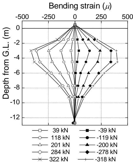
Figure 11 Distributions of bending strains down the pile shaft
