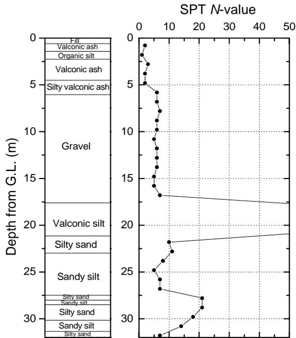
Figure 1 Profiles of soil layers and SPT  $N$ -values at Kiusu site
