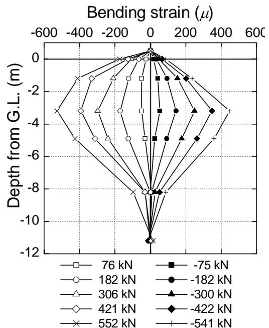
Figure 5 Distributions of bending strains down the pile shaft
