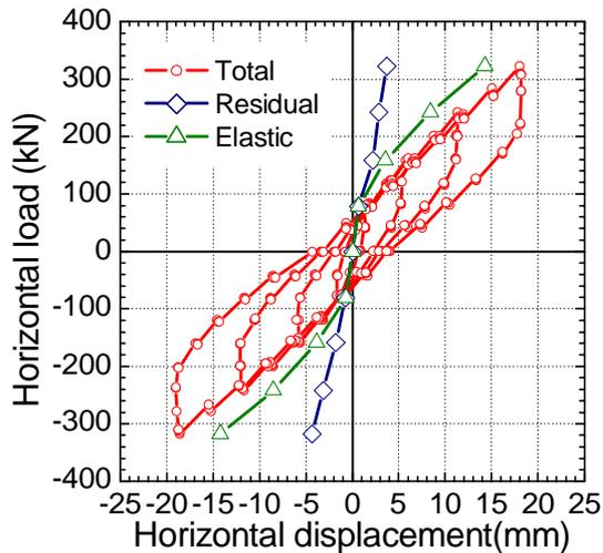
Figure 10 Horizontal load vs horizontal displacement in Shinotsu site
