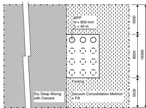
Figure 8 Soil improvements around abutment and piles
